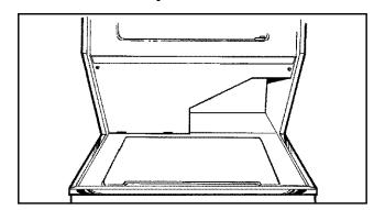
Lift access panel up until tabs at sides of panel slip out of slots at sides of dryer.
