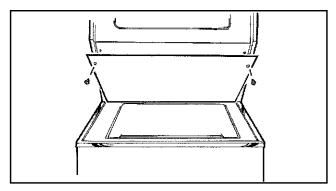
Remove two Phillips-head screws at top of panel.
