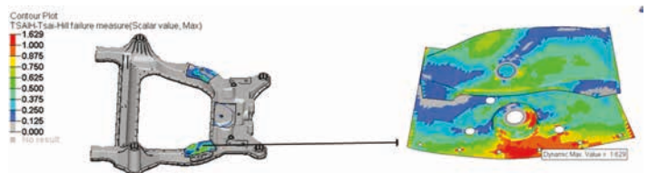
Figure 3: CAE predicted failure on control arm front joint laminate
