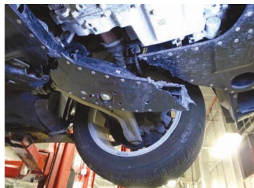
Figure 32: CF subframe – post vehicle special event test
