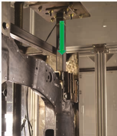
Figure 28: Strength test – control arm rear joint loading
