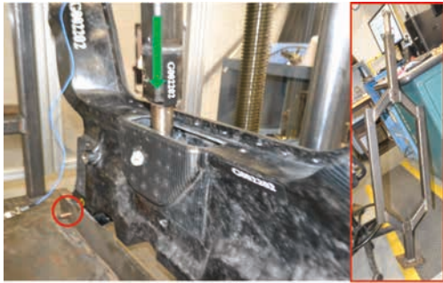
Figure 20: Strength test – roll restrictor loading
