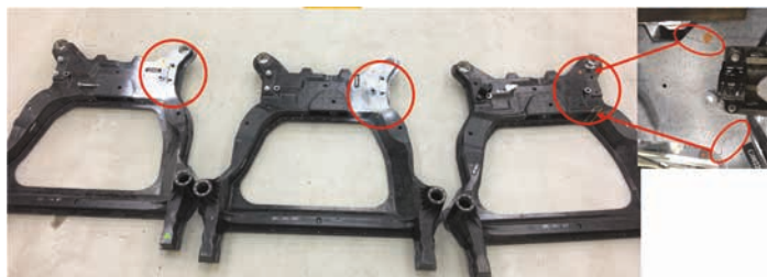
Figure 29: strength test – control arm rear joint loading damage
