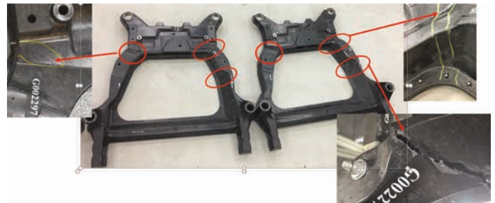
Figure 25: strength test – control arm front joint loading damage
