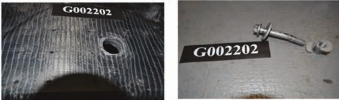
Figure 21: strength test – roll restrictor loading damage
