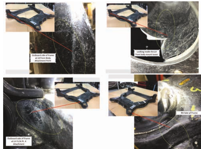
Figure 17: cracks - vehicle durability test
