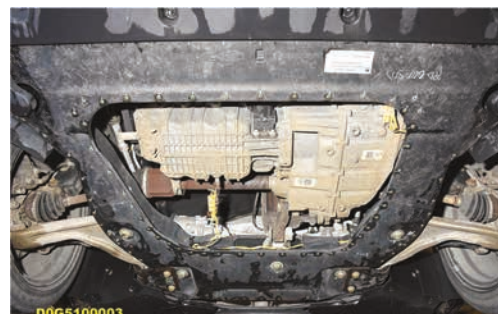
Figure 18: CF subframe - post vehicle durability test
