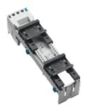
DIN rail adapters for components that have a 35-mm symmetrical DIN rail mounting provision. Available in 45-mm or 54-mm widths and 200-mm or 260-mm heights with one or two DIN rails. Most commonly used to add width to a powered EQUES EasyConnector for reversing contactor applications or to mount other components that are wider than 81 mm. The side-mounted module adds width to any adapter in 9-mm increments and maintains the IP20 fingersafe design of the busbar system.
