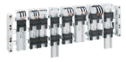
DIN rail adapters for components that have symmetrical DIN rail mounting provision. Additional DIN rails can be added to the adapter. Can be directly mounted on 12, 15, 20, 25, 30 x 5 and 10 busbars, and section busbars. EQUES EasyConnector is a trademark of Wöhner GmbH & Co. KG.
