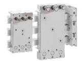
Adapters configured specifically for many of the industry's leading molded-case circuit breakers. The hole pattern for the mounting screws, pitch and length of the terminal connections are specific to the breaker they are designed to mount. Can be directly mounted on 12, 15, 20, 25, 30 x 5 and 10 busbars, and section busbars. *EQUES PowerConnector is a trademark of Wöhner GmbH & Co. KG.*
