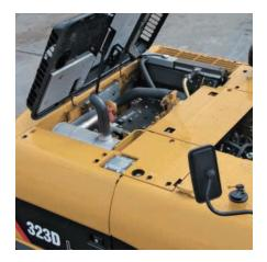
**Performance.** The Cat C6.4 with ACERT<sup>TM</sup> Technology offers more engine power, and runs at lower speeds for better fuel efficiency and reduced wear.
