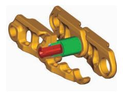
**Tracks.** The 323D comes standard with grease lubricated tracks. The track links are assembled and sealed with grease to decrease internal bushing wear, reduce travel noise and extend service life lowering operating costs.
