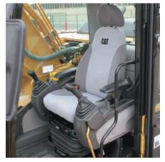
**Consoles.** Redesigned consoles feature a simple, functional design to reduce operator fatigue, ease of switch operation and excellent visibility. Both consoles have attached armrests with height adjustments.
