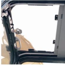
**Skylight.** A unique large polycarbonate skylight provides very good upward visibility, especially useful in above ground applications.
