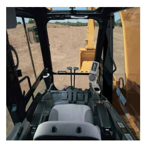
**Operator Station.** The workstation is spacious, quiet and comfortable, ensuring high productivity during a long workday. The air conditioner and attachment switches are conveniently located on the right-hand wall, and the key switch and throttle dial are on the right-hand console. The monitor is easy to see and maximizes visibility.
