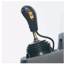
**Low Effort Operation.** Hydraulic joystick controls provide ease of lift and tilt functions. A single joystick is standard. An integrated directional control switch on the joystick provides easy operation and enhanced productivity. A two lever control is optional.
