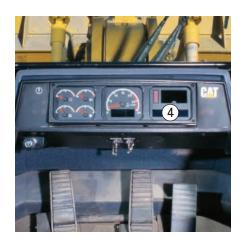
Vital Information Management System (VIMS). Is now standard. This system is a user friendly display system that provides operators and service technicians with information on the machine's major components and systems. (4) In the event that a problem occurs on the machine, the VIMS system gives pertinent information that leads to a more accurate diagnosis and a reduction of overall downtime.
