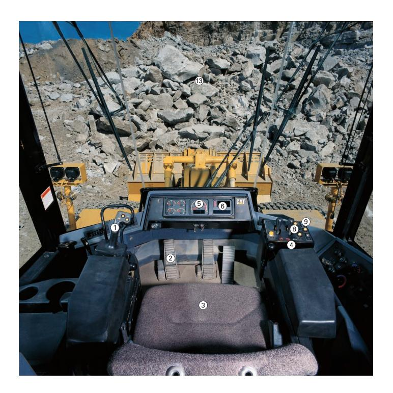
**Spacious Cab Design.** Incorporates innovations for operator comfort, maneuverability and productivity. Features include outstanding viewing area, excellent cab ventilation, interior sound levels below 75 dB(A), standard coat hook, cup holder, storage bin, intermittent wet-arm wipers, room for a large lunch cooler and radio-ready.
