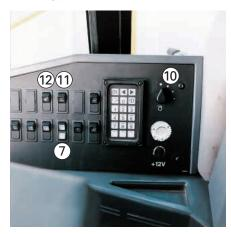
**Automatic Kickouts.** For lift, lower and bucket tilt are adjustable electronically from the cab. (7)
