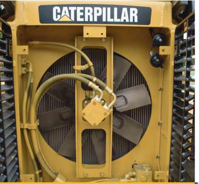
The engine radiator, Air To Air After Cooler (ATAAC), and hydraulic oil cooler are packaged in a single plane. Aluminum bar plate construction provides durability and allows for higher heat transfer and superior corrosion resistance. The standard cores feature 6 fins per inch to allow debris to pass through and reduce plugging concerns.
