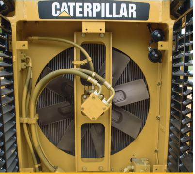
The engine radiator, Air To Air After Cooler (ATAAC), and hydraulic oil cooler are packaged in a single plane. Aluminum bar plate construction provides durability and allows for higher heat transfer and superior corrosion resistance. The standard cores feature 12 fins every 51 mm to allow debris to pass through and reduce plugging concerns.
