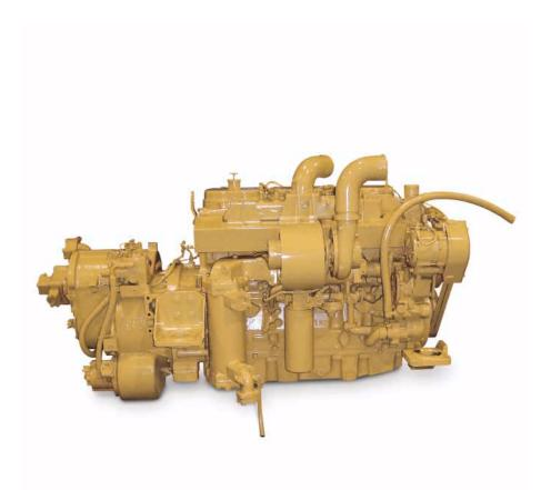
**Turbocharged and Aftercooled.** Air-to-air aftercooling provides improved fuel economy by packing cooler, denser air into cylinders for more complete combustion of fuel and lower emissions.
