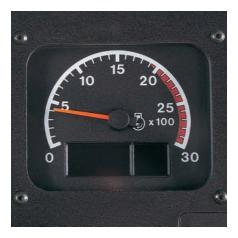
• Tachometer/Speedometer Module. Displays engine speed, ground speed, gear indicator, and machine direction.
