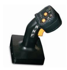
STIC™ Steering Control. STIC™ combines directional selection, gear selection and steering into a single lever for maximum responsiveness. Simple side-to-side motion turns machine right or left. Transmission shifting (forward/neutral/reverse) is controlled using a three position rocker switch. The thumb operated upshift and downshift buttons control manual shifting.
