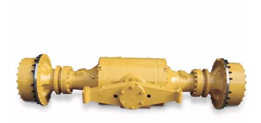
**Final Drives.** Cat final drives work as a system with the planetary power shift transmission to deliver maximum power to the ground. Built to withstand the forces of high torque and impact loads, double reduction final drives provide high torque multiplication to further reduce drive train stress.
