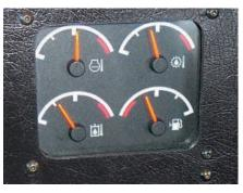
• **Gauge Cluster.** Maintains a constant display of vital machine functions, including: engine coolant temperature, transmission oil temperature, hydraulic oil temperature, and fuel level.
