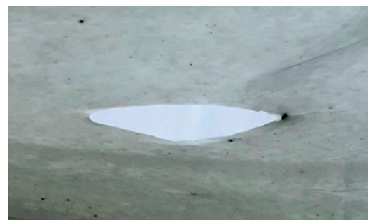
Typical pin hole in recycled film
