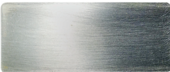
No corrosion as protected by acid scavenger
