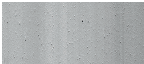
Magnification PE film surface showing the effect of 1000 ppm of a standard calcium stearate.
