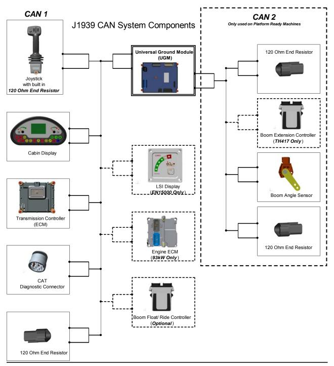
Figure 1 CAN bus component and control units' overview
