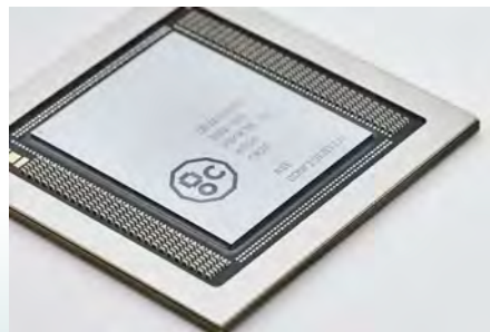
Graphcore's IPU chip has more than 1,200 cores. (Image: Graphcore)
