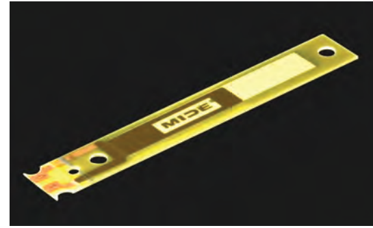
Figure 1: The S234-H5FR-1803XB piezo crystal converts vibrations into electrical energy. (Image: Piezo.com)
