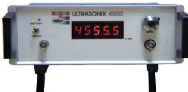
Fig. 6. Compressional wave velocity (P-wave) measuring device 'Ultrasonix 4600'
