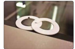
The laser-etching device is also capable of quickly and accurately cutting custom shapes, gaskets and spacers. With its cutting capabilities it makes an excellent addition to our rapid prototyping services.
