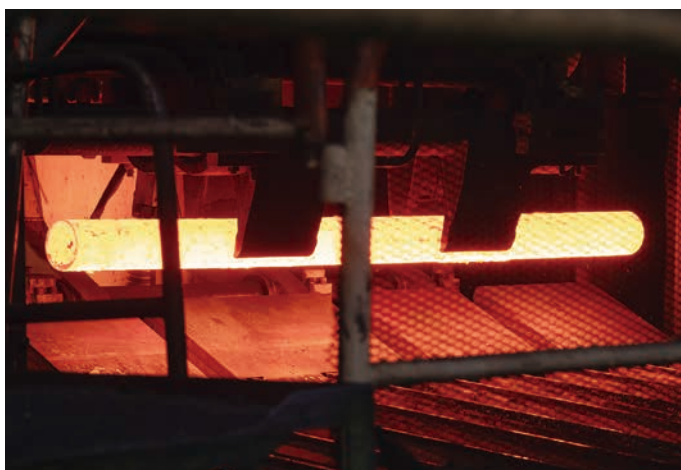
Rotary hearth heating furnace
