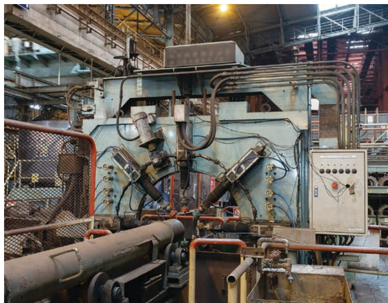
Ultrasonic automatic outside diameter and wall thickness measuring device
