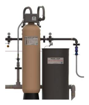
**Mechanics:** Requires tempered water. Electrical requirements for the *Digital Fleck Head* are 120 VAC from an uninterruptable, ground fault protected circuit. Drain must facilitate up to 50 GPM.
