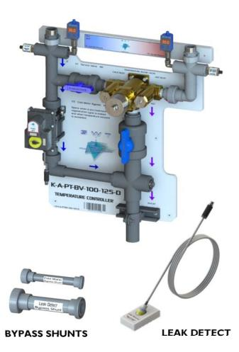
Provided in event of an electrical valve failure. Simply un-screw union nuts on electric valve and replace with bypass shunt until repairs are complete. **Mechanics:** Requires SWT Municipal City Boost System with SWT Pre-Treatment Monitor with 24VDC electrical. Inlet water piping capable of delivering 20 GPM both hot and cold, and between 30-100 PSI pressure.
