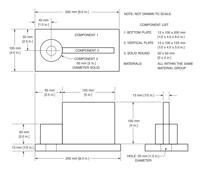
Figure 1—Test Specimen Components, Dimensions, and Layout
