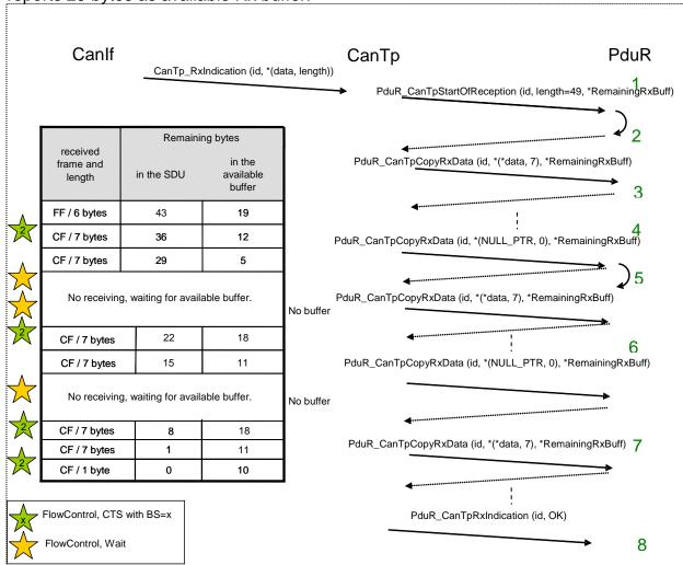
Figure 8: Example of receiving process
