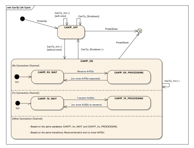
Figure 4: CAN Transport Layer life cycle
