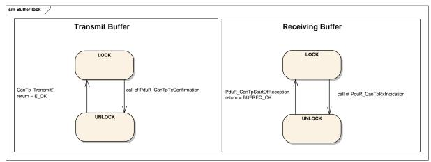
Figure 6: Tx and Rx Buffer locking
