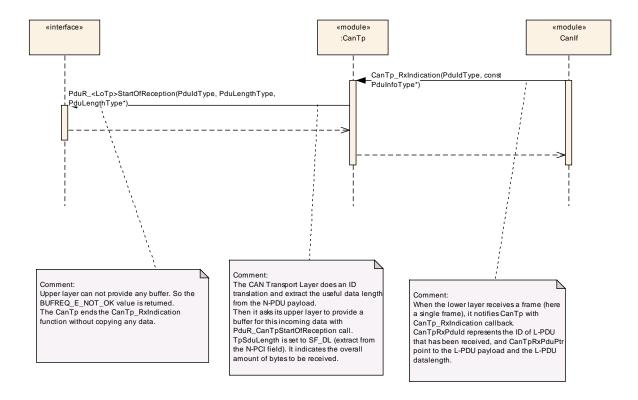
**Note**: This sequence diagram demonstrates the working of the CAN\_Tp module only. However, if the whole system is considered during such reception, more modules are involved. Since this reception can be triggered in the context of CAN ISR, the CAN\_Tp operation should be as short as possible.
