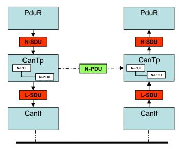
Figure 2: CAN Transport Layer interactions
