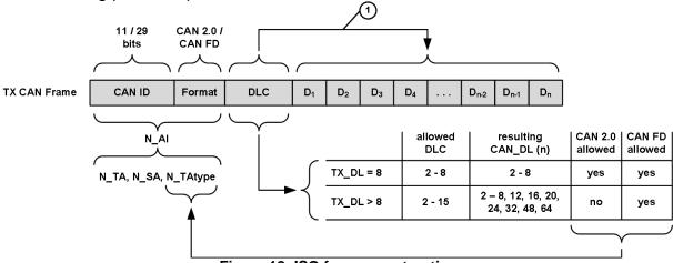
Figure 12: ISO frame construction
