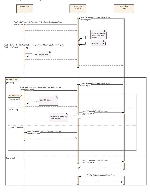
**Note**: This sequence diagram demonstrates the working of the CAN\_Tp module only. However, if the whole system is considered in such reception, more modules are involved. Since this reception can be triggered in the context of a CAN ISR, the CAN Tp operation should be as short as possible.
