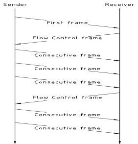
Figure 10: Example of multiple parts message
