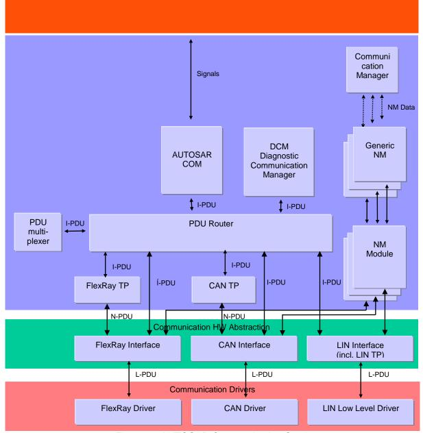
Figure 1: AUTOSAR Communication Stack
