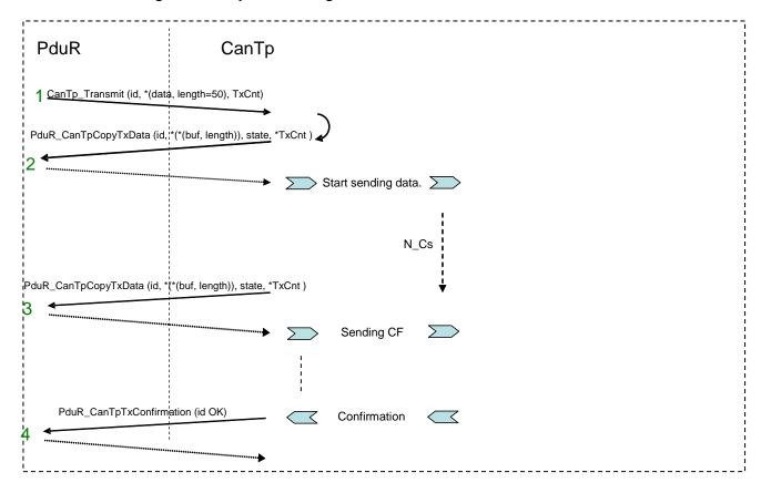
Figure 7: Example of transmit process
