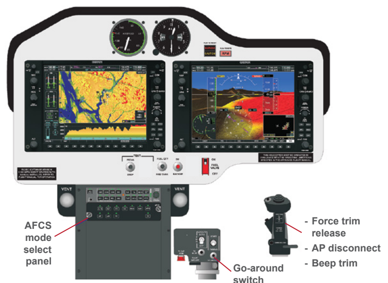
Bell 407GX i Flight Deck with Autopilot.
