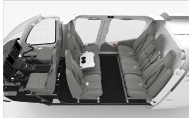
Six place club seating with 18.5" seats and one center seat fold down table.
