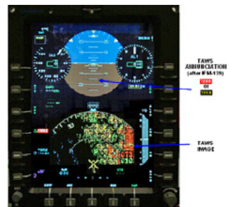
TAWS displayed as HSI underlay on PFD
