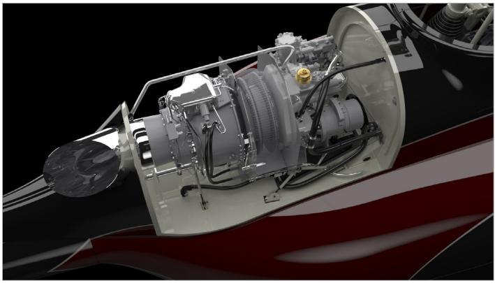
The Bell 505's Safran HE Arrius 2R Engine features a dual channel FADEC with automatic backup.
