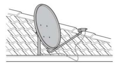
(a) A dish on the roof of a house guides the microwaves onto a receiver.Here are some statements about the signals picked up at the receiver.
