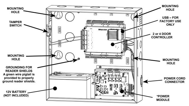
2 & 4 Door System Features and Mounting Locations (\*There are two types of power modules, one with lock power and one without)
