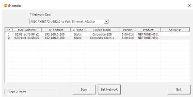
4. In this example, a server controller is located at 192.168.0.200 and client controller is located at 192.168.0.250. The client's IP address can be changed and the client can be
