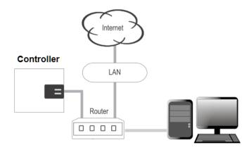
**NOTE:** LAN connection is only required for monitoring, reporting and configuration. Once the system is configured, it will operate without a LAN connection.
