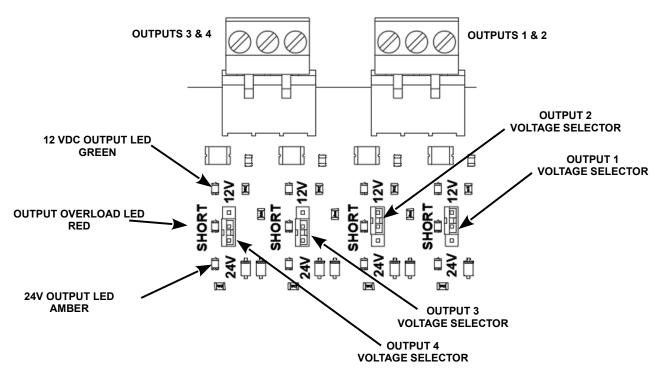
Power Module Output LED Indicators (only on models with with lock power)
