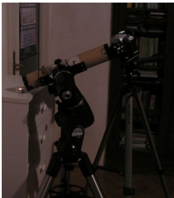
Fig. 1: A spectroscope with a camera, prepared to photograph a spectrum of a candle
