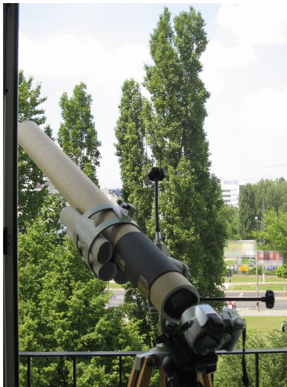
Fig. 6: Spectroscope with a camera prepared to photograph a spectrum of sunlight
