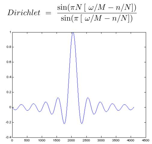
The bars are there because we chose a simple window -- instant on, instant off. The FFT of the window is a Dirichlet function. In short: the bars represent the FFT of the <u>window</u>, not the FFT of the empty space. This provides a powerful reason to take windows that aren't instant on/instant off.
