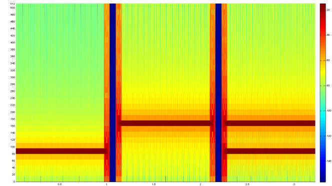
The window size is still 64, so it still sits inside the gap. But the overlap of windows is about 98%, and so the empty space is contaminated.
