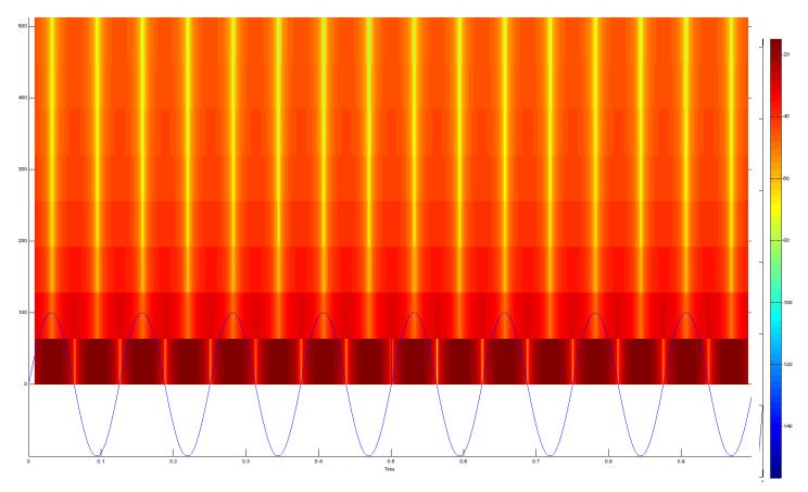
This is the "fine detail", in close-up, and the blue curve is my sine curve. Looking at it, it's tempting to think, 'wow! the spectrogram is picking out the individual peaks of the sine curve. Groovy! Unfortunately, red indicates power; yellow indicates significantly less power.
