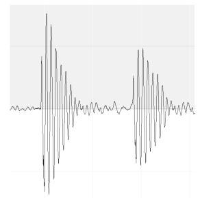
It's reminiscent of the artificial clicks we constructed in the Uncertainty supplement of Chapter Three. Those were characterized by a fundamental frequency -- which you can see as a dark band in the spectrogram -- followed by high frequency harmonics, but falling off slowly in power.
