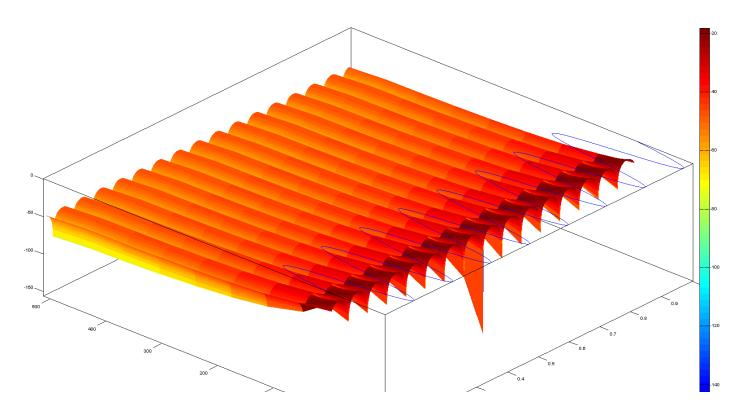
This is a good time to ask, 'what is going on here?' Start by following one frequency in the FFT. We've forced it into a window of length 16, so its real and imaginary components look like tiny sine or cosine waves.
