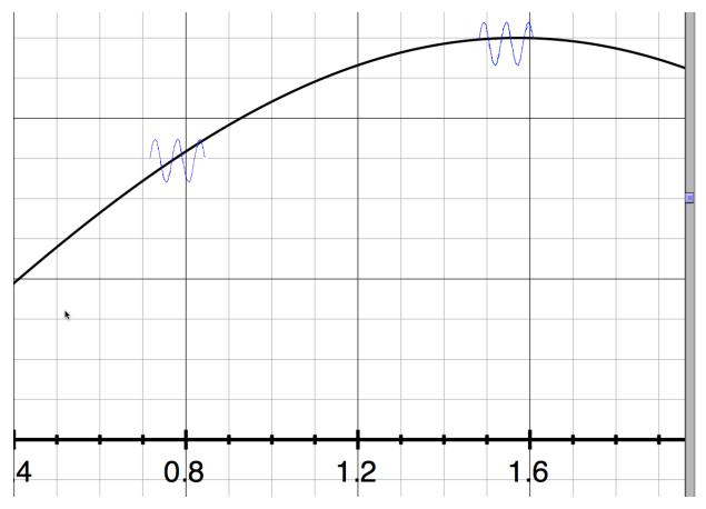
Here the little blue wave represents the exponential used in computing the power in the FFT. So: which of the two blue waves above give the greatest power? The way to compute the FFT is to multiply the exponential by the function, and integrate.
