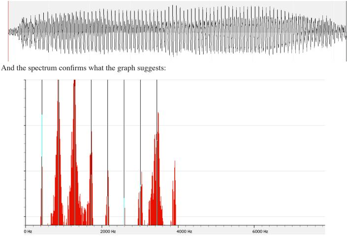
The spectrum consists of a fundamental and some fairly noisy harmonics. The reason for this has to do with the way the vocal tract produces vowels. Air is forced from the lungs, through the vocal folds, which vibrate and are
