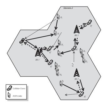
Fig. 1. Network model and sub-band sharing for a cellular network with D2D communications.
