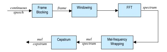
Figure 5.3 Block diagram of the MFCC processor
