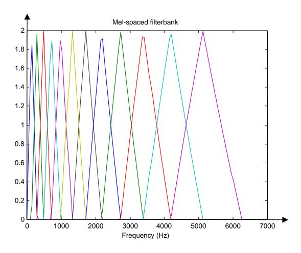
Figure 5.4 An example of mel-spaced filterbank
