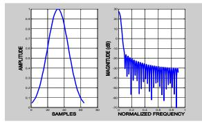
*Figure 2.1* : The time and frequency description of a Gaussian Window with " $\alpha$ =2.5"
