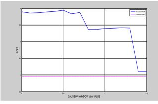
Fig. 2 (e) : Speech quality Objective Measures SEG-SNR and SNR Variation With " $\alpha$ ", (CAR-NOISE of 0dB SNR)
