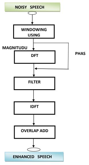
Figure 4.1 : Block diagram for Spectral Subtraction Algorithm
