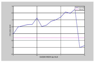
Fig. 2 (d) : Speech quality Objective Measures LLR and FSG-SNR Variation With " $\alpha$ ", (CAR-NOISE of 0dB SNR)
