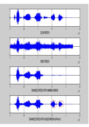
*Fig. 2 (a)*: Speech Signal Enhancement comparison  $(\alpha = 0.5, CAR-NOISE of 0dB SNR)$
