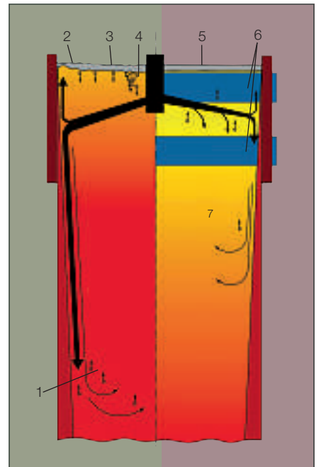
2 Flow in a continuously cast strand without FC Mold (left) and with FC Mold (right)
