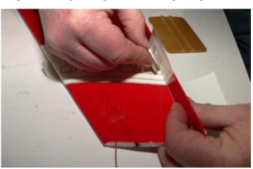
10. Carefully peel the backing off of the top of the graphic. Be sure to pull at an angle and horizontal to the graphic.
