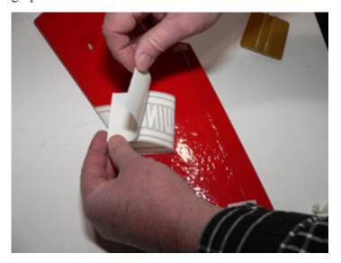
8. Press the rest of the graphic down working your way from the center of the graphic towards the back of the wing. Be sure to hold the elevon straight when applying the graphic.
