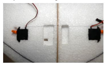
5. Install the rest of your radio gear. Make a shallow slit in the wing going the one wing tip and press the receiver antenna in the slit with your thumb nail. Leave the excess antenna dangle from the tip at this point.
