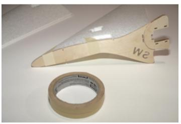
6. Glue the remaining wing to the motor mount using epoxy. Again, use masking tape to help hold the wing to the motor mount while the glue dries. Make sure the wing cores are in perfect alignment with the motor mount.
