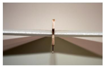
7. Insert the motor into the motor mount. You will need to mark where the motor fits into the mount and cut a small amount of foam out of the wing so that the motor can slide all the way forward.
