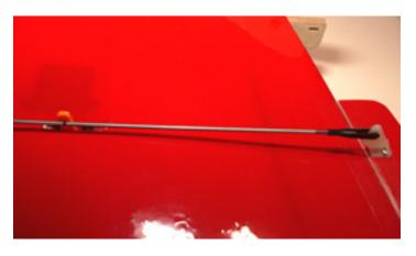
10. Make a Z-Bend in the pushrods where you marked them using a Z-Bender or a small pair of pliers. Cut off the excess pushrod and attach to your servos.
