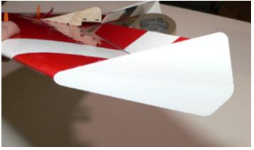
7. Using a straight edge, mark the location of the 1/2A control horns on the elevons.
