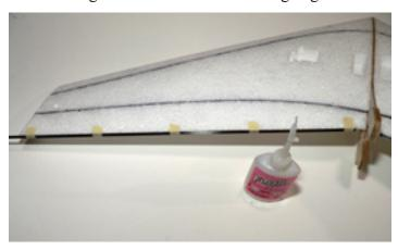
10. Now put a piece of wax paper on your flat work surface. Place the trailing edge of the wing flat against the work surface and glue the CF Flat to the trailing edge with Thin CA. You can use a small amount of CA Accelerator to speed up the drying process.
