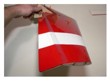
3. Tape the underside of the elevon to the wing while the elevon is flipped up.
