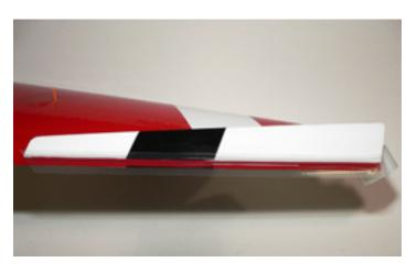
4. Find the coroplast tiplets. Now make a mark from the tip of the tiplet to the back. You will glue the tiplet to the wing with this line on the centerline of the airfoil. Sand the tiplet where it will be glued to the wing.
