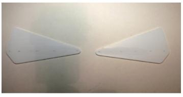
5. Glue the Right tiplet to the elevon using medium CA and CA accelerator. Use the marks on the tiplets as a guide to align them properly.
