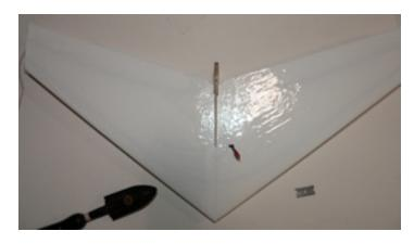
4. Now cover one side of the top wing. Using the same technique as before, iron the edges down, making sure to overlap the bottom covering by 1/2". Trim excess.
