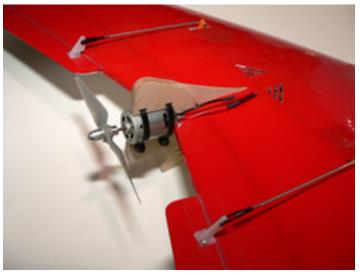
12. Cut the covering off of the cooling holes in the speed control cover. You can cut them off of the receiver cover as well, but it isn't necessary.
