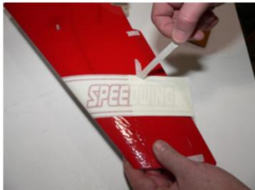
7. Now peel the rest of the transfer backing off of the graphic.
