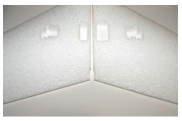
5. Glue the mount to one wing core with 5-minute epoxy. Use just enough epoxy to cover the root of the wing. To help hold the wing in place, use a couple of strips of masking tape.
