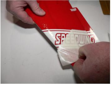
11. Carefully go over the top of the graphic again to make sure all the edges are stuck to the covering.
