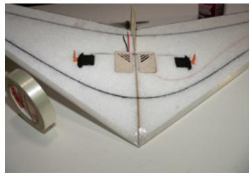
9. Find the two elevons. Sand a 45 degree angle on the leading edge of each elevon. Make sure you make a right and a left elevon. Also, lightly bevel the underside of each elevon. This will make the wing faster as you will need less reflex to fly (up elevator).
