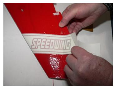
9. Bend the elevon up and cut the graphic along the hinge line using a sharp X-acto or single edge blade.
