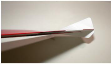
6. Make a small hole on the inside of the left tiplet and pull the antenna through the hole into one of the corrugated flutes. Now glue the left tiplet on with med. CA. Run the antenna back and forth through the tiplet flutes leaving a few inches hanging out of the back of the tiplet.
