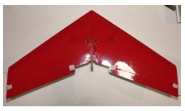
10. Iron on any design you'd like. I use racing stripes on most of my wings as they show up very easily when the wing is at high speeds and at a distance.
