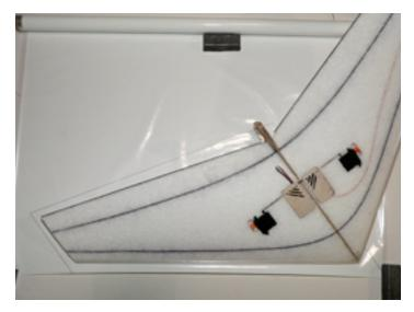
2. Use low heat settings on your iron and iron the covering to the center of the wing. Then stretch the covering and iron it to the tip of the wing. Now, stretch the covering and iron it to the leading and trailing edges. You will shrink the center of the covering after you cover the whole wing. Trim excess covering.
