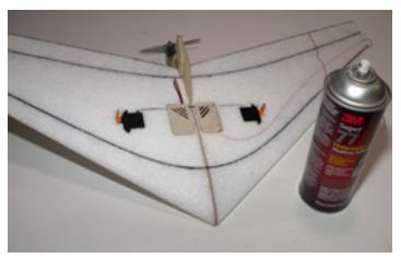
8. Place a strip of strapping tape along the leading edge of the wing. The strapping tape helps prevent the leading edge from becoming damaged when hitting sharp objects.
