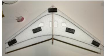
7. Now flip the wing over and lay the wing in the top beds. Repeat previous steps 2-6. Be sure to weigh down the wing so that it remains flat when gluing in CF Flats.
