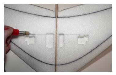
4. Place some servo tape on the bottom of the servos and place the servos in their precut pockets. Also, make a small hole in the speed control pocket for the battery connector to fit through.
