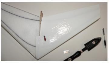
3. Now cover the other side of the bottom wing using the same covering technique. Make sure to overlap the center of the wing by at least 1/2". Trim Excess.
