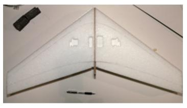
4. Using a sharp X-acto knife or single edge blade, make a single cut along the lines that you have marked. Only cut as deep as the CF Flat is wide. I find it helpful to use a little bit of masking tape on the blade so that I don't cut too deep.
