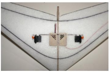
7. Now use some masking tape to cover the motor mount. Spray a light coat of 3M77 spray on the top and bottom of the wing.
