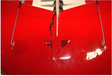
13. Use industrial strength Velcro to attach the battery. It is a good idea to cut the covering out from under the Velcro and attach the Velcro directly to the foam with some medium CA. Also, glue the 1/32" ply connector plate to the wing and the battery connector to the connector plate using medium CA.
