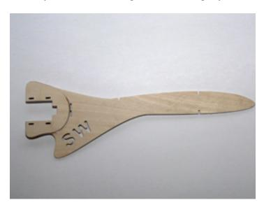
3. Now place the mount along one wing core and mark where the ply doublers come in contact with the foam. This foam will have to be cut from the cores so that the motor mount can be glued flush to the cores.
