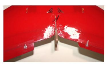
9. Connect a pushrod to the control horn and hold the elevon level. Mark the pushrod where it goes over the servo control horn. (Note: I use the second hole from the top on the elevon control horn and the second hole from the bottom on the servo horn).
