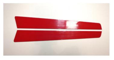
9. Now temporarily tape the elevons to the wing using a couple of strips of masking tape. I do this so that any stripes/details I put on top of the base covering can be ironed to the elevons as well.
