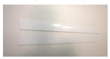
8. Now cover the top of the elevons making sure to overlap the bottom covering. Check for warps in the elevons and use your iron to shrink one side of the covering or other to take the warp out.
