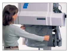
With the touch of a button, the SpeedyPacker® system quickly dispenses an Instapak® foamfilled bag.
