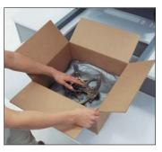
The product is placed onto the foam-filled bag as it expands in the carton, forming a custom-fit cushion.
