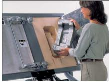
The operator removes the custom cushion that is ready to package and protect your product during shipping and handling.
