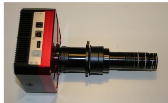
Fig. 3: Grism, distance rings and ATIK One camera.
