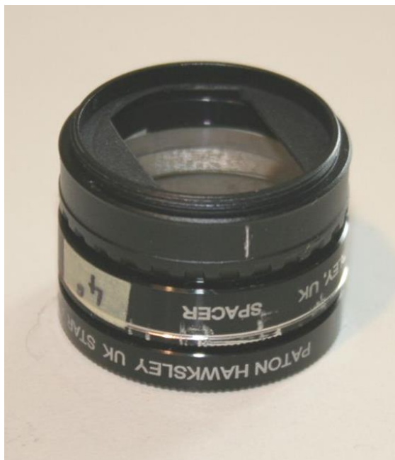
Fig. 2: Grism Setup: 16mm field diaphragm, 4° Thorlabs Prism, Star Analyser 200.
