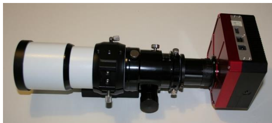
Fig. 4: Setup of grism, ATIK One and ED 60/330 mm.
