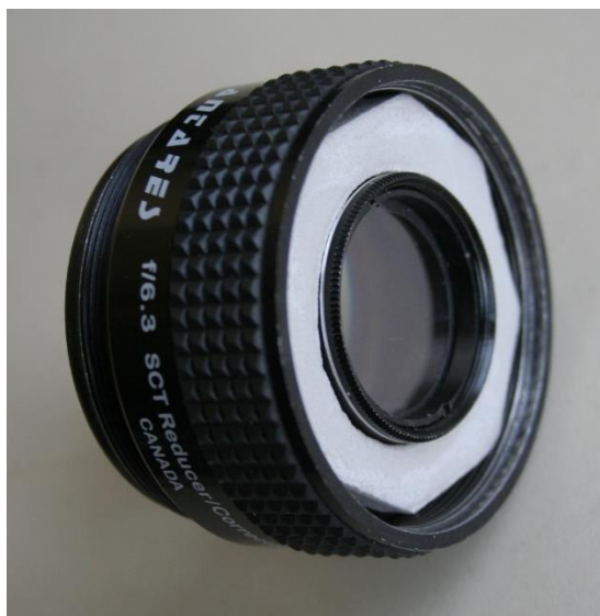
Fig. 5: Star Analyser mounted in front of focal reducer.
