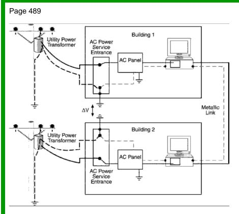
Figure 9F-4—Example of intersystem ground noise between different buildings
