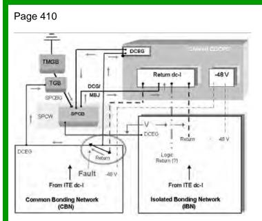
Figure 9-70—Undesirable dc paths due to the Return of the ITE in the CBN not properly bonded to the SPCB
