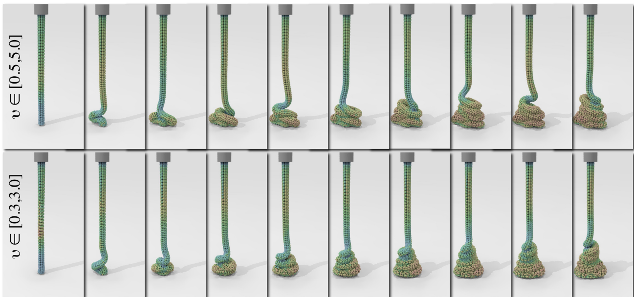
Fig. 7. Jet buckling with different viscosity intervals. Our method provides different coiling effects varying the parameters of Cross model.
