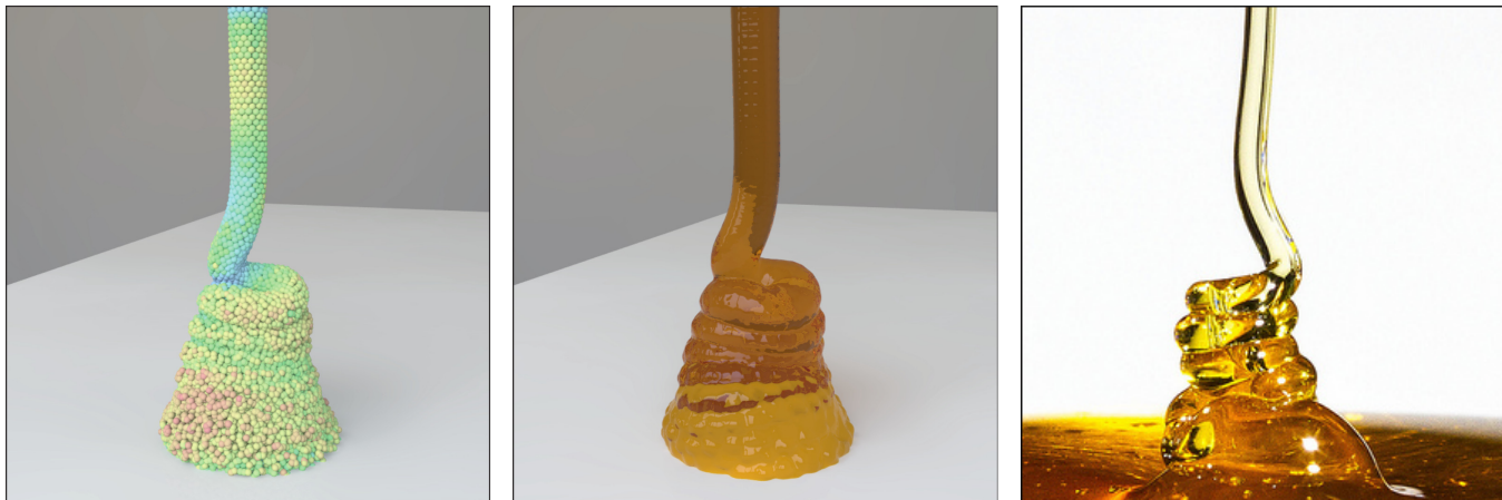
Fig. 1. The liquid rope coiling effect: our technique with SPH fluid particles (left), and the respective free surface (middle) and a real image of honey coiling (right) extracted from Flickr repository.
