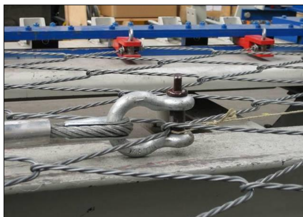
Left: Standard test for the determination of tensile strength per running meter
