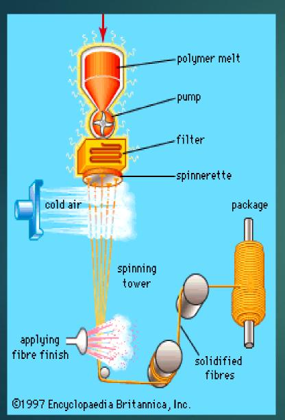
Feeding (Polymer chips) Melting Metered extrusion Cooling and solidification by cold air Moisture conditioning Lubrication Yarn driving Packaging
