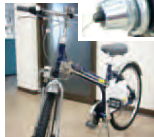
2WD Bicycle by SHESCO KSB Bevel Gears are used in the driving components in both the front and rear wheels.
