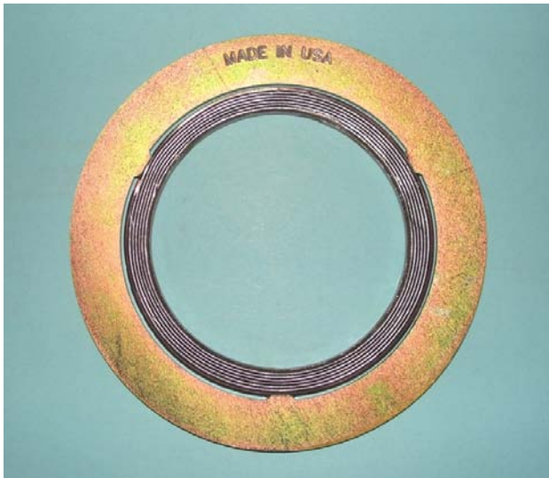
Figure 15 Spiral wound gasket with anti-buckling, controlled-density windings and filler, and low-stress-to-seal construction (Note: no inner ring required)
