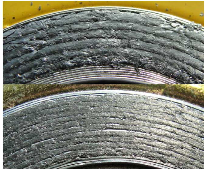
Figure 13 Variation in winding density for the same size and pressure class spiral wound gasket - NPS 1 x 150 Manufacturers “A” (top) and “Z” (bottom)
