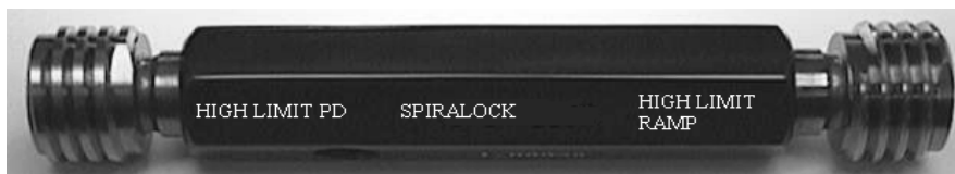
NOT-GO Pitch Diameter and Ramp Gage
