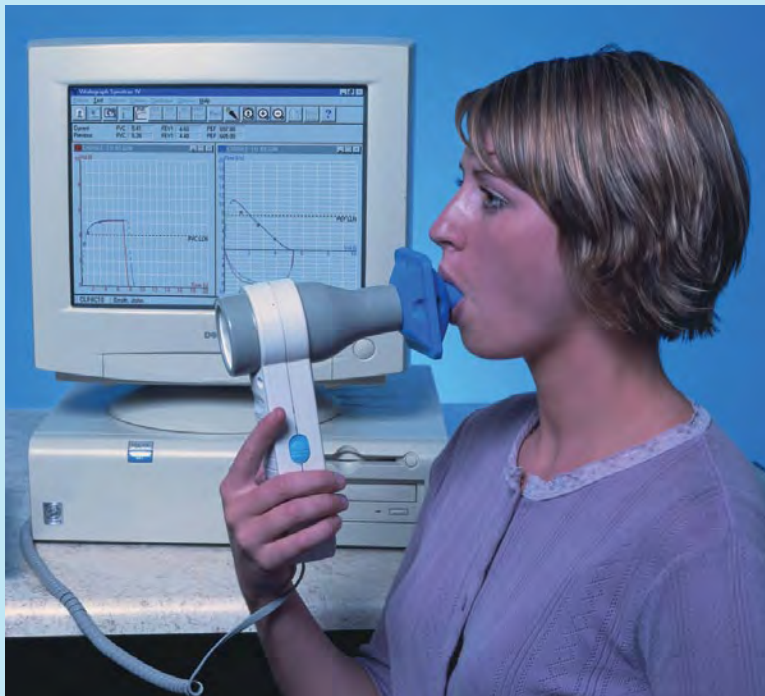
Figure 3. Example of a flow spirometer sensor with mouthpiece, filter, and real-time display.
