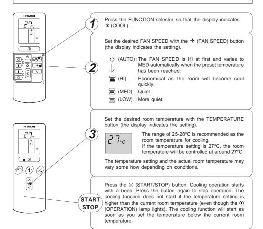
■ As the settings are stored in memory in the remote controller, you only have to press the ① (START/STOP) button next time.
