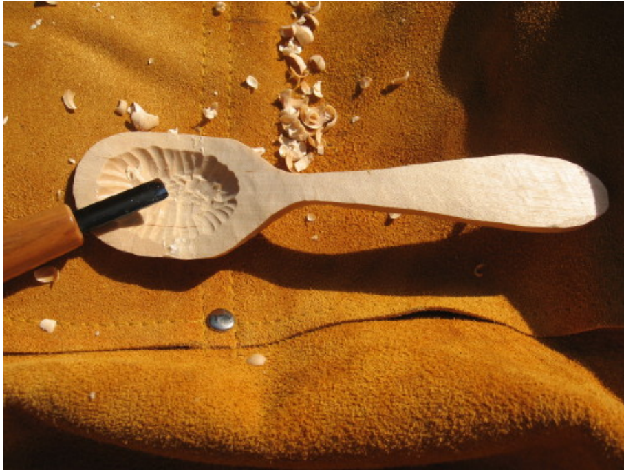
Step 5c. Initial hollowing is complete Now this is ready for the spoon knife.
