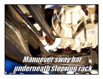
» Once the sway bar is removed, install your new Hotchkis sway bar in the same manner as removal. See diagram below for proper orientation.
