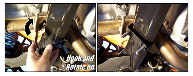
» Once the brackets are positioned, you may secure them to the beam using the supplied clamp plate and hardware.
