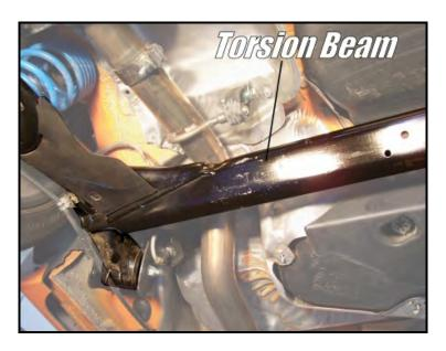
As a brief summary, the 2 bearing mounts will be installed on the straight section of the torsion beam. The end links will attach to the lower shock mount.
