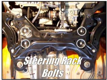
» Now, remove the 4 large bolts that secure the subframe cradle to the body using a 21mm socket. The subframe should droop down slightly. The subframe droop down slightly (5-6 inches), but it might fall rather quickly, so be careful.
