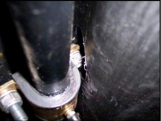
» For aggressive racing applications, H-Sport suggests spot welding the torsion beam brackets to the torsion beam. See picture for weld locations. Make sure to grind and clean any surface that is to be welded to insure proper cohesion and penetration.
