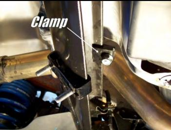
» Lube and install the polyurethane bushings onto the sway bar. Rotate the sway bar up toward the torsion beam. Install the bushing bracket and secure with the provided washers and nuts. Fully tighten.
