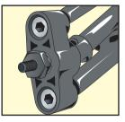
You should not adjust the top pivot ball; unscrewing it will increase positive camber and will also change the wheel's toe-in.
