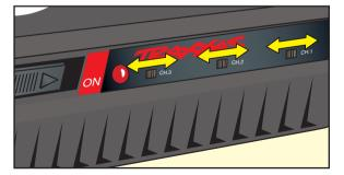
Remember, always turn the TQ-3 transmitter on first and off last to avoid damage to your SportMaxx.
