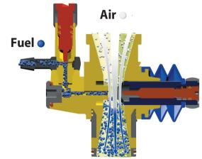
To help provide a better understanding of engine tuning and why it's necessary, the following is a brief explanation of the air/fuel combustion process that takes place inside the engine.
