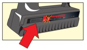
**4.** Turn on the transmitter and check the power indicator for a solid red light.
