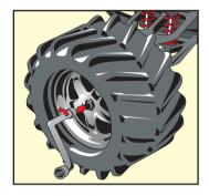
1. Remove a wheel from the SportMaxx using the larger (8mm) end of the glow plug (universal) wrench.
