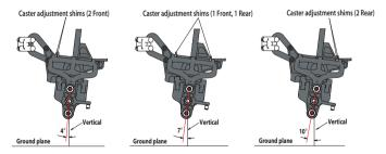
The stock caster setting is 7-degrees with one shim at each end of the arm. Reduce the caster angle to 4-degrees by removing
