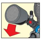
body. With the base removed, the foam element is visible in the bottom of the filter body. Pull out the foam element.
