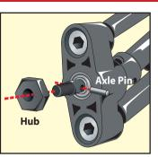
**4.** Reinstall the wheels, making sure none of the axle pins have fallen out from behind the hex hubs.
