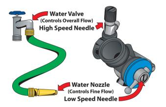
pulled completely away from the needle seat leaving it fully open. At that point, fuel metering is entirely controlled by the high-speed needle. Again, using our water hose example, when the spray nozzle at the end of our garden hose is fully open, then the main water valve can be used to adjust how fast the water flows.
