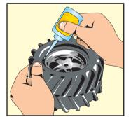
**2.** Use your thumb to push the side of the tire away from the rim. Place one or two drops of CA glue into the opening and release the tire. Capillary action will draw the glue around the bead of the tire.
