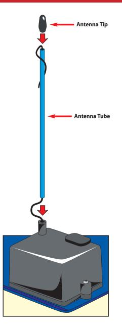
Spray a little window cleaner on the antenna wire to make it easier to push through the antenna tube.
