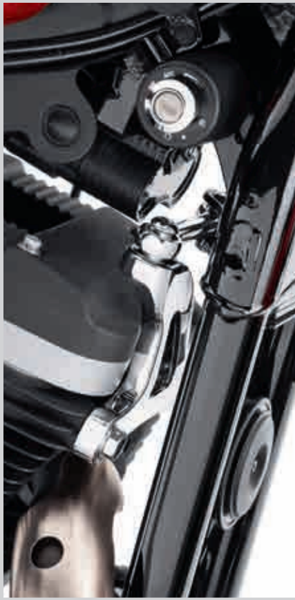
FRONT ENGINE MOUNT BRACKET AND STABILIZER LINK
