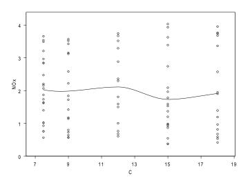
Figure 3.37: Compression ratio versus nitrogen oxide in the ethanol data set (default smoothing).
