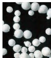
0 50 100μm Powder generated by DL410
