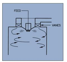
Figure 8: Cyclonic flow (fast mixing)
