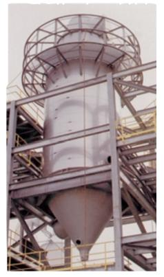
This spray dryer uses pressure nozzles although the slurry is very abrasive. The tight particle size distribution was required to improve quality and energy efficiency of a downstream process.
