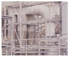
These quad cyclones are recovering product after chamber bottom separation. A venturi scrubber was used for emission control.
