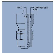
Figure 2: An example of a two-fluid nozzle
