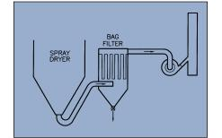
*Figure 10: An example of single point bag filter collection*
