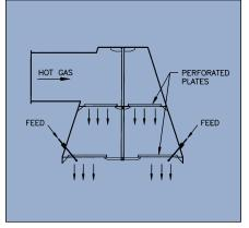
Figure 7: Parallel flow (slow mixing)
