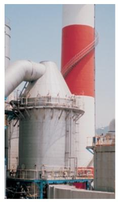
can eliminate the need for sizing/classification equipment when the product average particle size is less than 500 microns. "Nondusting" powders can be made which is beneficial for hazardous products, animal feeds, dyes, and other products.
