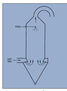
Figure 5: Counter-current flow
