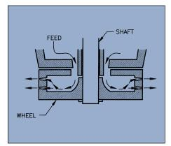
Figure 3: An example of a centrifugal atomizer
