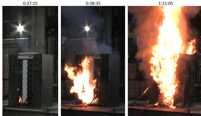
Photos of LFP fire development during large-scale free burn test: near time of ignition (left), near time of predicted sprinkler operation (middle), peak heat release rate (right).
