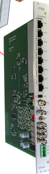
CTF Trigger and Clock Fanout in SRS slot 9
